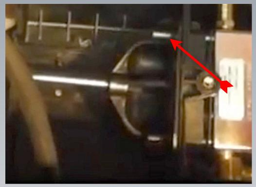
THIS IS GOING TO BE THE DIFFICULT PART, INSTALL THE SPACER
